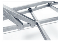
Hot-dip galvanized chassis
