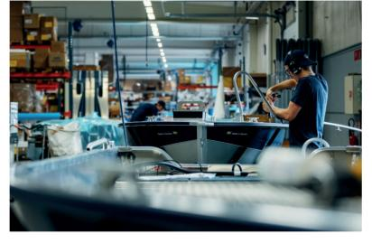
around a form. This form produces the familiar, soft and harmonic lines that constitute one of our trademarks. This forming technology saves energy because it tempers most of our aluminium alloys. Consequently, the sheets do not need to be heat hardened.
