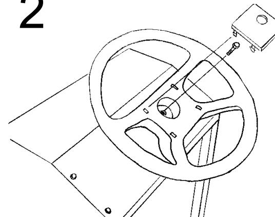
Unscrew the bolt on top of the console (where the steering should be). Put the steering wheel in proper position and fasten the bolt. Place the black plastic cover in the centre of the wheel.
