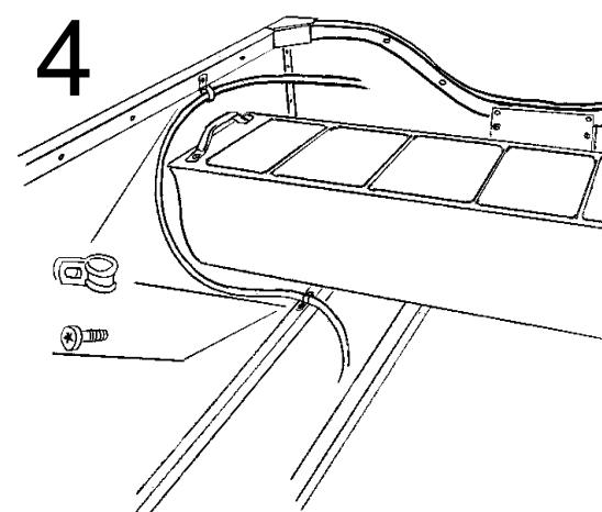
Fasten the steering cable to the gunwale and the reinforcement profile using the enclosed clips. Use the existing screw on the gunwale and drill a hole (4,5 mm) in the reinforcement profile and use a M5x16 screw to fasten the clip.
